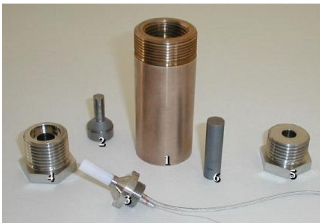
Figure 1. main construction of the CC33 nonmagnetic optical pressure Cell, 1 - Body, 2 - Piston, 3-Obturator, 4 - Screw for piston, 5 - Screw for obturator, 6 - Push rod. [2]
