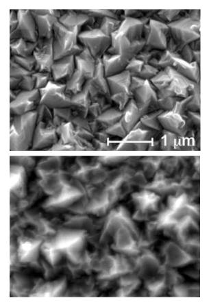
**Figure 3:** Surface morphology of a 1.8  $\mu$ m thick LP-CVD ZnO film, grown on glass (top) and on a microcrystalline bottom cell (bottom). Image size approximately 4 x 3  $\mu$ m<sup>2</sup>.
