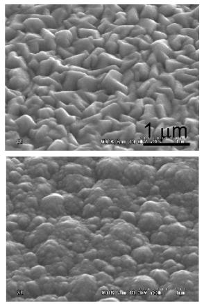
**Figure 1:** Surface morphology of the Asahi-U substrate covered with the Ag/ZnO reflector (top) and after deposition of a 4  $\mu$ m thick microcrystalline bottom cell (bottom) [14]. Image size approximately 4 x 3  $\mu$ m<sup>2</sup>.
