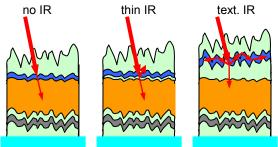
Figure 2: Illustration of intermediate reflector concepts in n-i-p micromorph tandem cells. From bottom to top, the layer stack consists of glass\text. SnO<sub>2</sub>\Ag\ZnO\ $\mu$ c-Si cell\ X \a-Si top cell\text. ZnO front contact. Here, X represents the intermediate reflector which is, from left to right, either absent, thin, or thick and textured.
