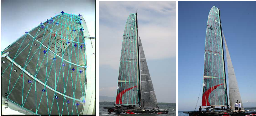
Figure 4.17: Modeling the deformations of a main sail by minimizing an objective function under constraint. The black circles in the leftmost image are targets that can be automatically detected and were used to establish correspondences with the reference configuration. The algorithm can estimate the 3D deformations at a rate of approximately 10 Hz on a standard PC.
