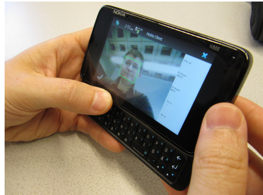
Figure 1. A capture of the MOBIO face and speaker authentication demonstration system running on the Nokia N900.
