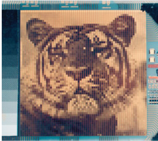
Figure 1.10: Organic display for monochrome imaging on a rigid glass substrate. Image reproduced from [57].
