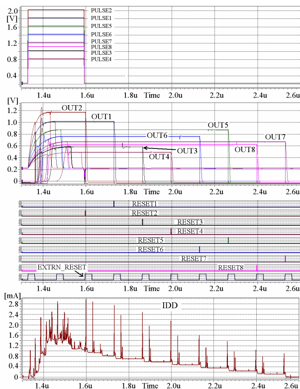
Fig. 10. Postlayout simulation results of the pulse shaping block together with a peak detector
