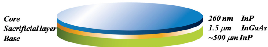
Fig. 3.2.3. InP wafer cross section.
