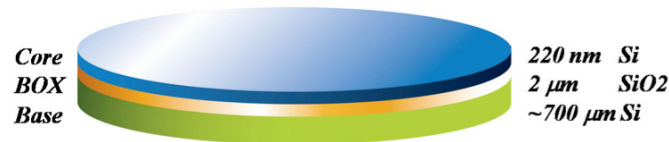
Fig. 3.2.1. SOI wafer cross section.
