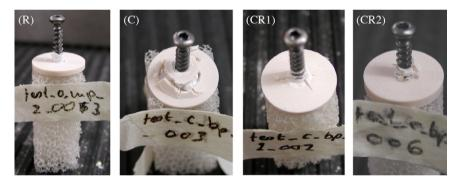
Fig. 2. Failure modes were defined qualitatively based on visual criteria: mode R, resin disk breaks; C, cement breaks at screw surface; CR1, mode C+cracks appear in resin disks without failure; CR2, mode C+resin disks thread break without crack propagation.
