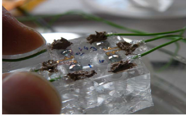
Figure 9.7. A completed device with a set of four membranes, which can be used as three lenses and one actuator, or one lens and three actuators. For scale, two fingertips are visible on the left.
