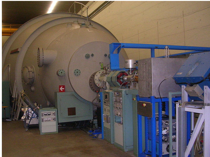
Figure 3.4. Van de Graaff generator integrated with a particle accelerator*.
