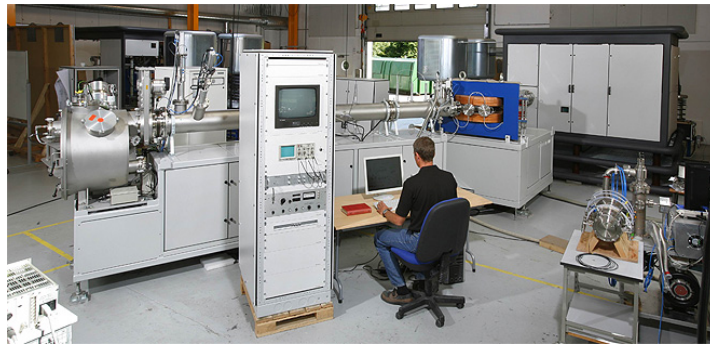
Figure 2.11. 200 keV Ion Implanter – Danfysik Model 1090 *. High current ion source model 921A which operates in gas, vapor or sputter configuration, to produce ions from virtually any element in the periodic table.
