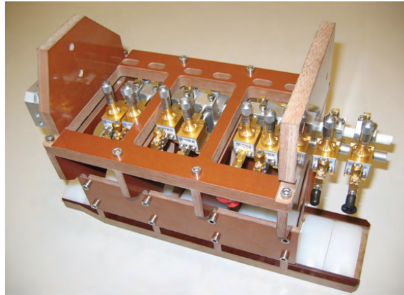
Fig. 3.3.3 Detector and focussing lens assembly for the FIR polarimeter diagnostic. There are 2 detectors and 2 lenses for each of the 5 beams crossing the plasma.
