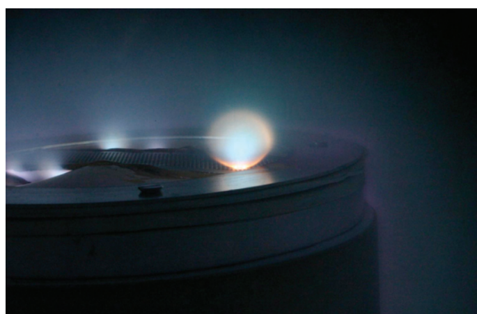
Fig. 2.6.3 Close-up of a hollow cathode in the arcing testbed.
