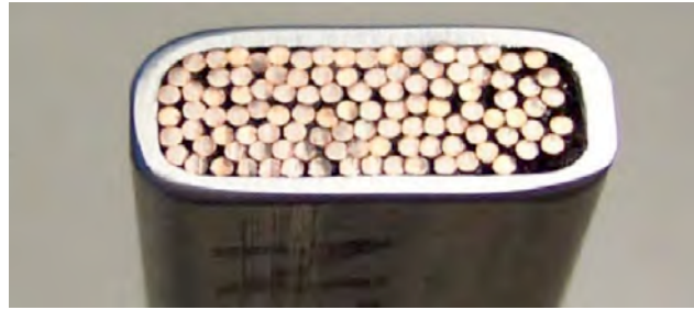
Fig. 2.5.9 Photo of a short piece of the rectangular cable-in-conduit conductor.
