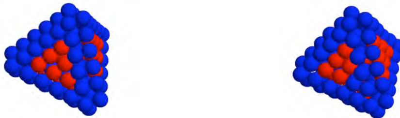
Fig. 2.4.2 Resulting atomic configurations, showing a stacking fault tetrahedron, following annealing of a 15 vacancy-triangular platelet at 800K for 3ps. Left: pure Ni, right: Ni containing 5at.% Al. Red atoms: hcp-coordinated atoms, blue: non-fcc, non-hcp, non-bcc atoms.
