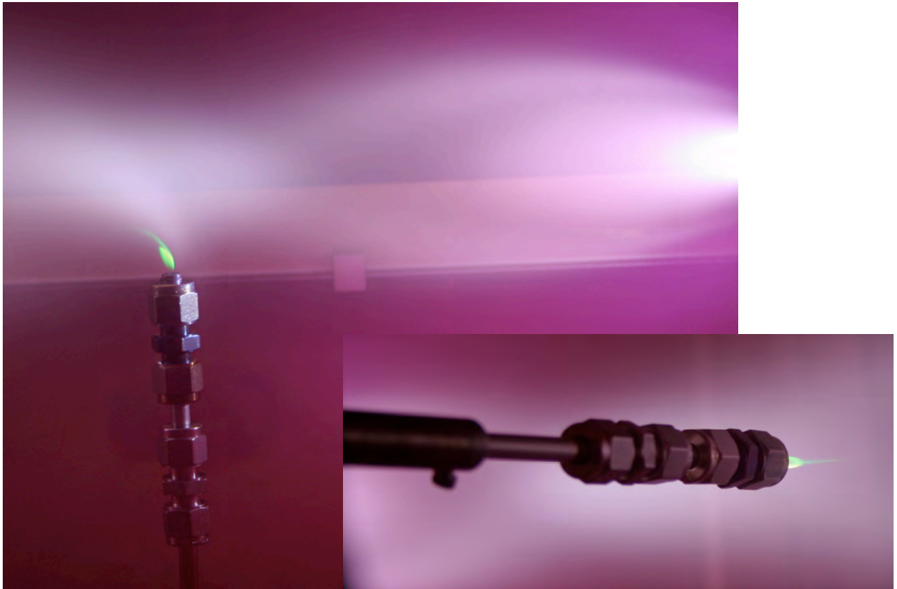
Fig. 2.6.3 Injection of Kr into the plasma jet generated by a F4 Sulzer Metco torch.
