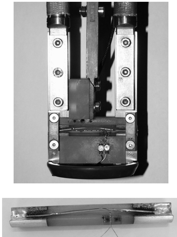
Fig. 2.5.14 Sample holder for short length, straight strand and (bottom) a strand extracted from a cable, soldered to the Cu/glass-epoxy supporting cylinder
