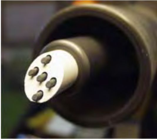
Fig. 3.2.11 The reciprocating Langmuir probe head following modification in early 2002. The 5 graphite pins are 1.5mm in diameter and mounted in a boron nitride (BN) insulating base, itself protected by a graphite housing. The BN base has diameter 10mm. The probe head is positioned by a slow drive and then reciprocates over a stroke of 15 cm on a fast timescale (~200ms) driven by a pneumatic system under 4bar of helium pressure.
