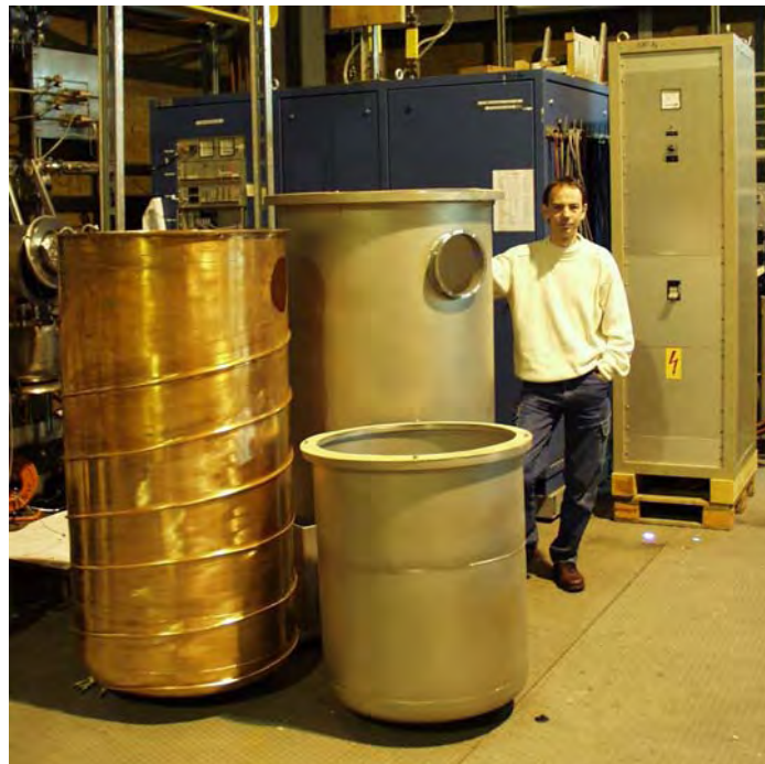
Fig. 3.6.3 Vacuum chamber, copper shield and He container before final assembly
