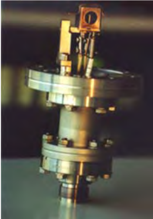
Fig. 3.2.12 One of the two ASDEX type fast ionisation gauges (this one is installed under the lower floor tiles) on its mounting flange.
