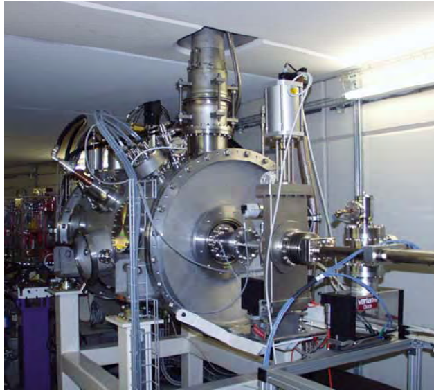
Fig. 3.6.4 The SUPER-3HC cryomodule installed in the SLS ring
