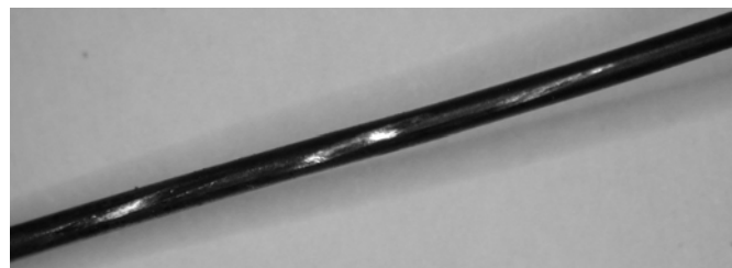
Fig. 2.5.17 Friction imprints (bright spot) at the strand crossovers, observed only at strands extracted from the high load section, o.d. =0.82mm.
