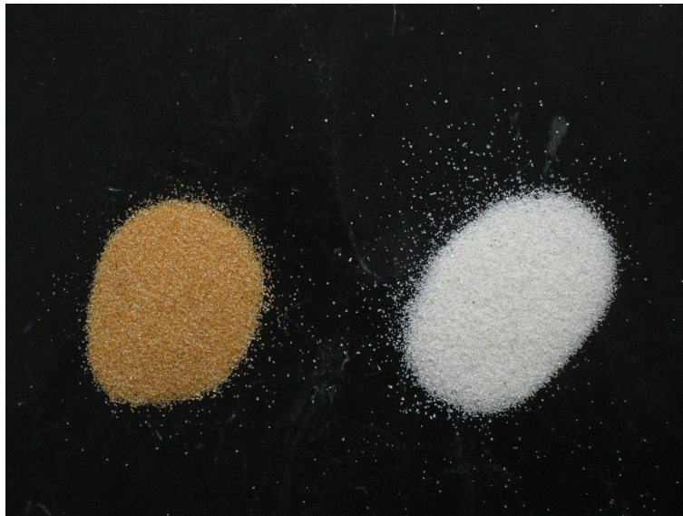
Figure 3.1: Iron oxide coated sand (left) and uncoated acid washed sand(right).
