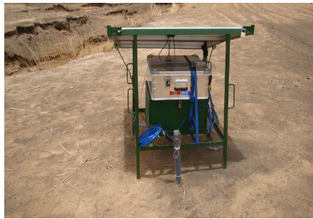
Figure 2.3: Start of DTS in the valley (see figure 2.2). The blue coil of the optical fiber is visible.
