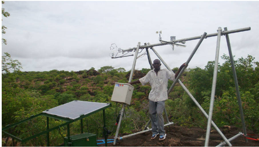
Figure 2.1: Energy balance (EB) station. This station is located on a hill
