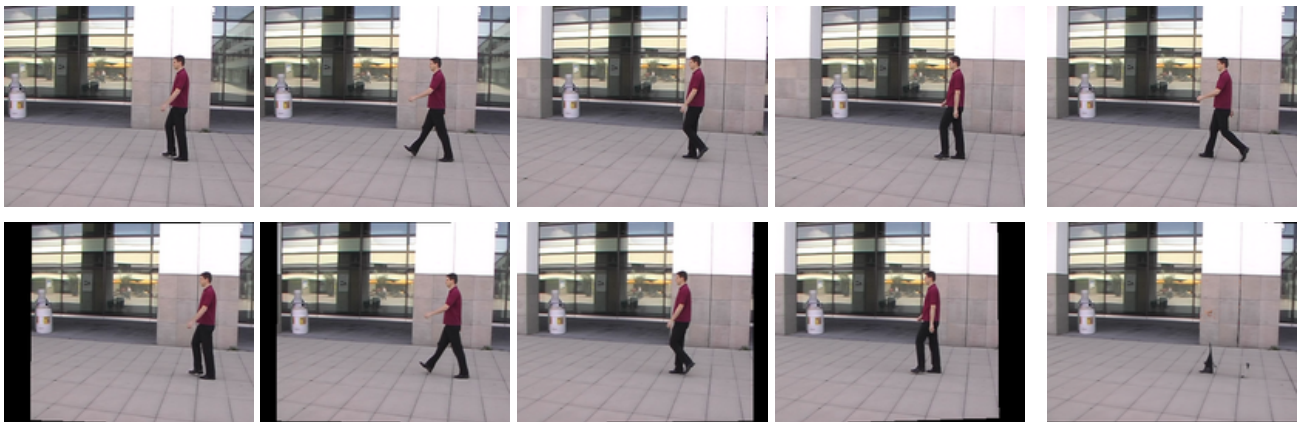
Fig. 11. Synthesizing a background image. First row: The rightmost image is the reference image whose background we want to synthesize. The other 4 are those before and after it in the sequence. Second row: The same four images warped to match the reference image. Computing the median image of these and the reference image yields the rightmost image, which is the desired background image.
