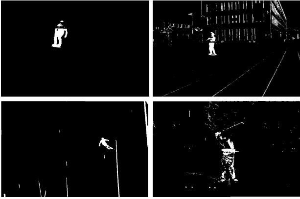
Figure 2. Input silhouettes used to compute our results. The silhouettes were extracted using a standard background subtraction technique on skating and golfing examples, while on skiing an intensity threshold was used.
