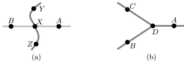
Fig. 3: Two cases that can lead to reconstruction errors. (a) A crossover with a single sample point that can be used to build either the horizontal \overline{AXB} branch or the vertical \overline{YXZ} one, but not both. (b) If there is no sample point at the bifurcation D , incorporating both the \overline{AB} and \overline{AC} paths into the graph will result in counting twice the pixels in \overline{AD} . This is avoided by introducing a sample point at D .
