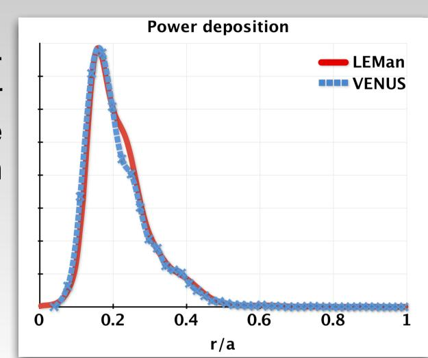
$T_{\parallel}^{H} = T_{\perp}^{H} = T_{th}^{D} = T_{th}^{e} = 5 \text{keV}; \ n_{e} = 4e19 \text{m}^{-3}, n_{D} = 0.99 n_{e}, n_{H} = 0.02 n_{D}; \ R_{0} = 3 \text{m}, a = 1.04 \text{m}; \ B_{0} = 3.45 \text{T}, B_{c} = 3.24 \text{T}, \beta = 1.3\%$
