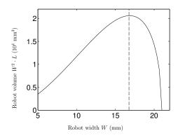
Fig. 4. Volume of one module depending on its width, the length being dependent on the width so that the module can pass bendings (Fig. 3).
