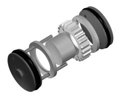
Fig. 5. Magnetic wheel construction without central axis to increase the holding force. The wheel has a diameter of 12 mm and a width of 10 mm. It holds 2.5 N with the rubber seals.
