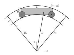
Fig. 3. Module length L and width W constraint.
