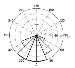
Fig. 10. Success of bend passing in %. 0, 90, 180 and 270° correspond to respectively up, left, down and right bends respectively. The bending has a 150 mm radius. Only upward bends are passing well, the robot is easily blocked in the other ones.
