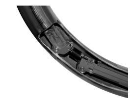
Fig. 8. Robot passing a curve going up.
