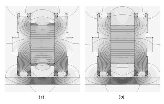
Fig. 6. 2D simulation of the version a and b of the magnetic wheel on a ferromagnetic plate. Changing the small supports for the magnets in non ferromagnetic material increases the force by 12% (from 2.26 to 2.5 N), as they introduced leakage.
