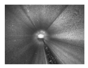
Fig. 13. View of the camera inside a clean 22 mm of diameter tube.
