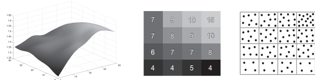
Figure 12: Blending the sampling rate at the patch boundary. Left: Continuous sampling rate. Middle: Discretized area weighted sampling rate. Right: Resulting sampling pattern.
