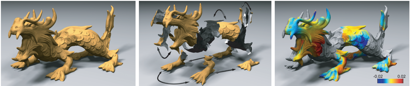
Figure 1: Symmetry detection on a sculpted model. From left to right: Original model, detected partial and approximate symmetries, color-coded deviations from perfect symmetry as a fraction of the bounding box diagonal.
