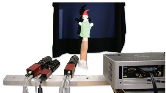
Figure 4: Our real-time structured light scanner based on active stereo delivers high resolution input scans from a single view.
