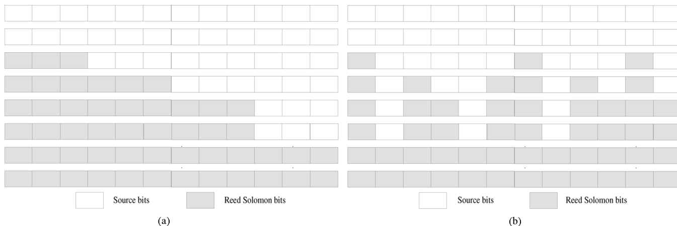
Fig. 2. Conventional structure of (a) is converted to block with interleaved columns in (b). If the symbols in the most protected columns are always fully recovered, they can serve as determinate information during the subsequent LDPC decoding.
