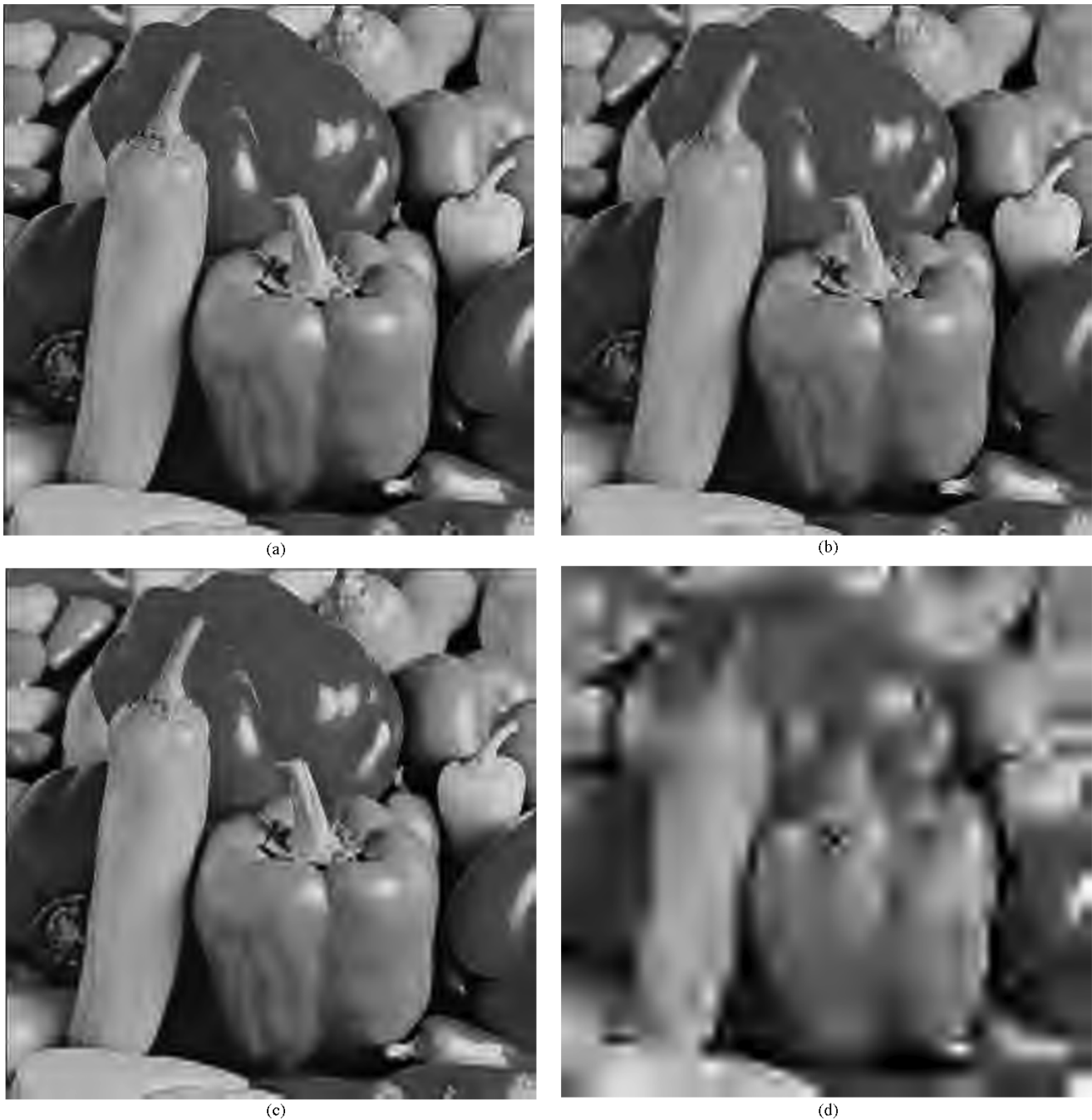
Fig. 15. Visual comparison for the “Peppers” image using the proposed method and the method in [4]. The optimization conditions were \overline{\text{SNR}} = 10 dB and f_D = 10^{-5} for both methods. Comparison in terms of average quality: (a) Proposed scheme (27.86 dB). (b) Sherwood method [4] (26.87 dB). Comparison in terms of a random transmission (the images were transmitted and decoded using the exact same simulation of the channel). (c) Proposed scheme (27.65 dB). (d) Sherwood method [4] (20.18 dB). It should be noted that the performance difference between the two methods would be much more pronounced for transmission in channel mismatch conditions.
