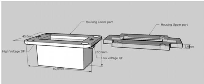
**Figure 10 The two housing parts. Lower part (left) made in PEEK and upper part (right) made in metal.**
