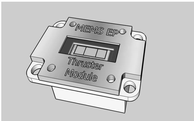
**Figure 5** A preliminary design of a miniaturized thruster module, including all main functions except the power supply and control unit.
