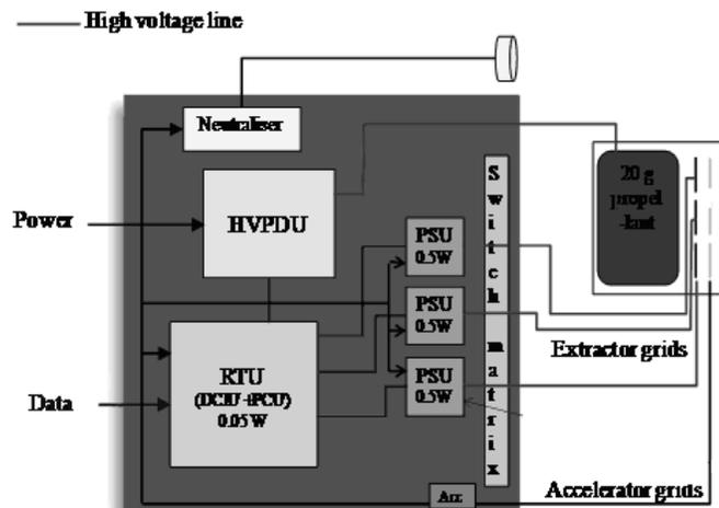
Figure 13 Potential implementation of MEMS EP cluster. CubeSat 1U, 1 module case.
