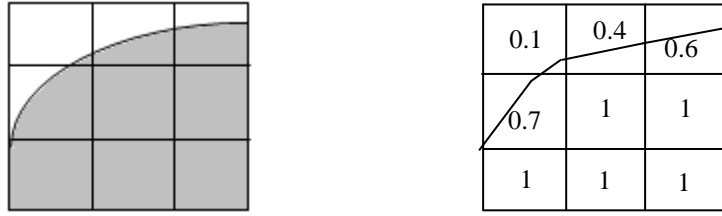
Fig. 1. Free surface approximation using the VOF method. Left panel shows the actual interface between the air and water phases, while the right panel represents the volume fractions associated with the interface using the VOF technique.
