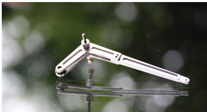
Figure 2.9: Structurally optimized main leg
