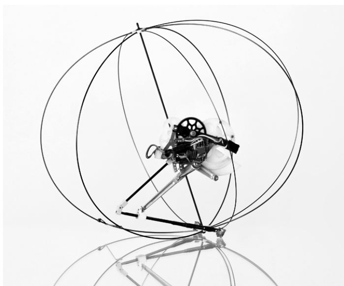
Figure 3.1: EPFL jumper v2, able to jump, land safely, upright and jump again. The cage has a diameter of 12cm (picture: Alain Herzog, EPFL)
