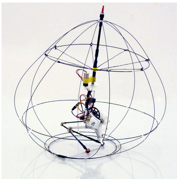
Figure 4.1: EPFL jumper v3 weighting 14.3g. The cage has a height of 18cm and allows the robot to upright itself after landing, steer and jump again
