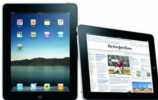
Figure 1.1: The I-Pad computer, released in April 2010, sprawling a 1 GHz processor, a 64 Gb storage and the mass of 680 grams.
