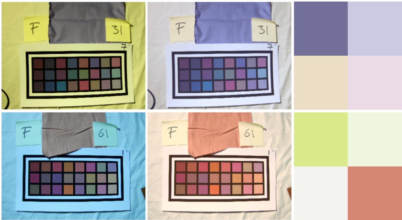
Figure 9. Paint samples are grouped together in palettes of four colors. The application matches the object color to one of the paints and returned the corresponding palette. The figure shows, from left to right, the uncorrected image, the corrected image, and the corresponding paint palette.
