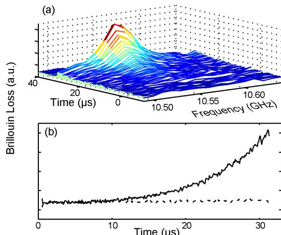
Figure 2 a) Brillouin loss spectra of the B-OTDA pump amplified in a FOPA. b) Traces of the probe Brillouin loss when the FOPA pump is ON (solid curve) and OFF (dashed curve)
