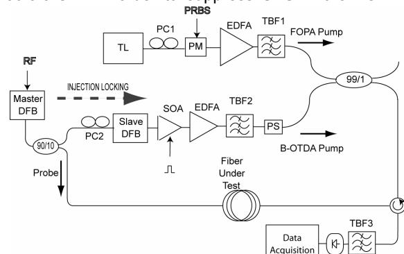
Figure 1 Experimental Setup. TBF: tunable Bragg filter, PM: phase modulator, PC: polarization controller
