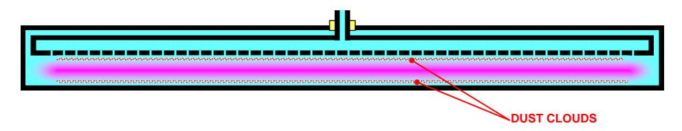
For a-Si:H deposition (amorphous Silicon), uniformity is mostly ruled by the dust cloud uniformity. Most important is Temperature uniformity. Indeed thermophoresis would push the dust cloud towards the cold side
