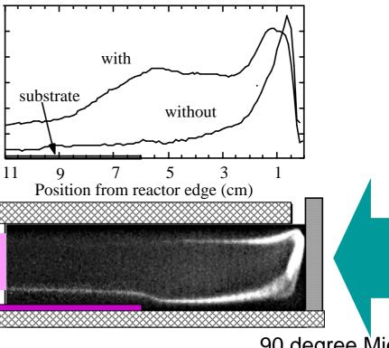
90 degree Mie scattering of a laser sheet
