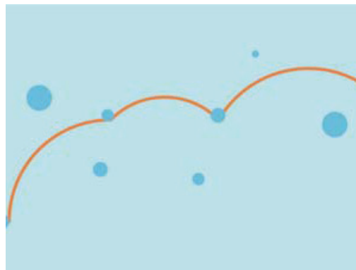
Figure 1.1 In crystals, the obstacles (blue spheres) are arranged in an irregular pattern. The orange line represents a pinned dislocation. Taken from Ref. 6
