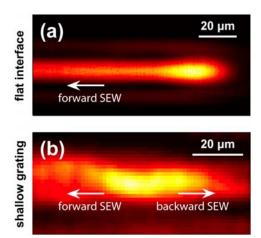
**Fig 1** TE-polarized near-field intensity map of surface electromagnetic waves: (a) at the flat interface of a multilayer, (b) at the surface of the some multilayer covered with a subwavelength dielectric grating. In (b), the field is acquired at a band edge.
