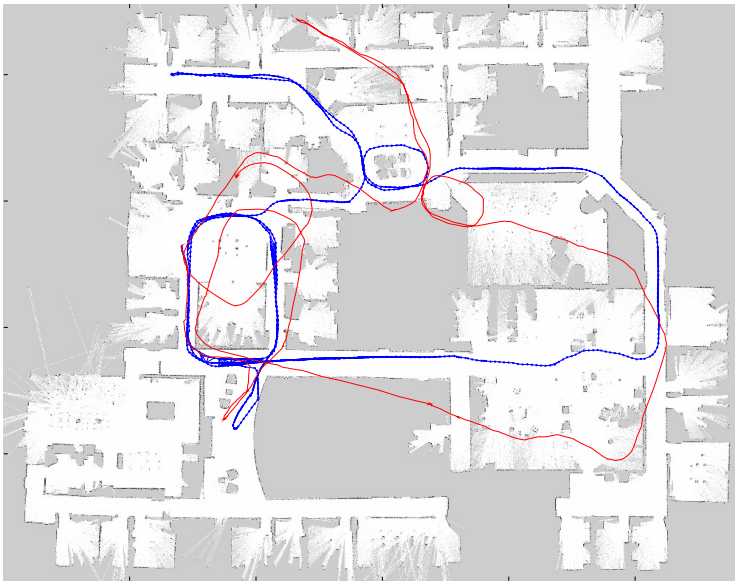
Fig. 5: Top: representative scenes from the large office loop, showing matched features in green. Note blurring, people, cluttered texture, nearly blank walls. Bottom: resultant skeleton graph (in blue) of 628 nodes and 1275 edges, overlaid on a laser map of the building. For comparison the VO trajectory without view match correction is shown in red. On the right is a closeup showing the matched views on a small loop. The optimizer has been turned off to show the links more clearly.
