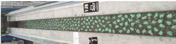
Figure: 1 Un-structured block-ramp
