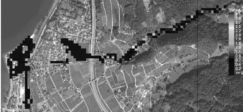
Figure 8. Maximum channel and floodplain water depth for HQ100 maximum with the proposed mitigation measure.
