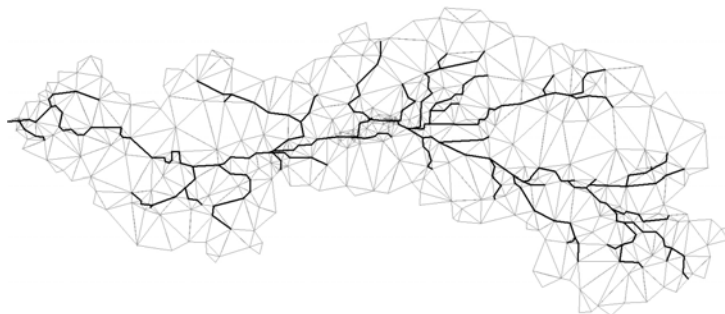
Figure 2. Domain decomposition showing triangle elements and simplified river network.
