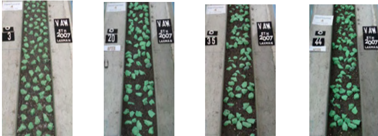
Figure: 10 Changes of blocks position after the discharges of 3, 20, 35 and 44 l/s
