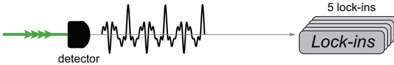
Figure 3.3: (Color online) Detection systems involving one detector. The signal from the detector is sent to 5 lock-in amplifiers.
