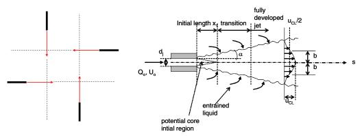
Figure 3 Left: Top view of a jet configuration with in black the nozzles and in red the middle axis of a starting jet's trajectory in an idealized case of no influence of the neighboring jets. Right: submerged turbulent jet.
