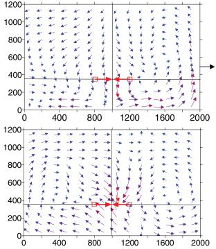
Figure 7. Above: Measured flow pattern in the longitudinal axis with the water intake at the right edge (level 500 mm, arrow). Below: Measured flow pattern in the transversal sense through the rotation axis of the jets. Units in mm. jet configuration with d = 8 mm, v = 2.8 m/s.
