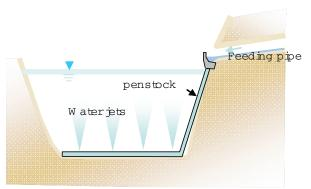
Figure 1. Schematic view of the water jets supplied by the feeding pipe coming from water transfer tunnels
