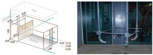
Figure 2 left: Schematic view of the physical model, right: a configuration with the four stiff sanitary pipes, the jets and the water intake in the background.
