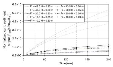
Figure 6. Normalized cumulated sediment output through the power intake in function of time. The dependency on the jet Froude Number and on the jet's plane level becomes visible.
