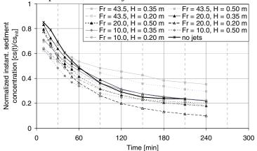
Figure 5. Normalized instantaneous sediment concentration in function of time. The dependency on the jet Froude number as well as the influence on the level of the jet's plane becomes visible. "no jets"-line: experiment with no jets, but with an evacuating discharge equivalent to the experiment with jets Froude number 10, the evacuated water compensated from the back wall.
