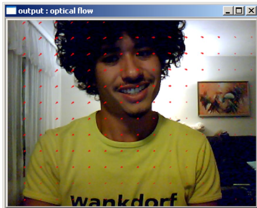
Figure 6.7: The optical flow for a bending head—input taken on the fly from webcam.
