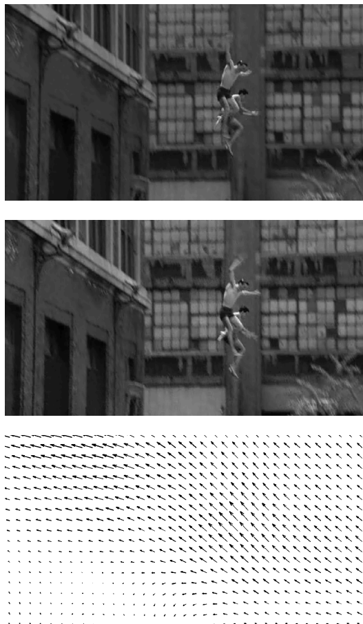
Figure 3.2: Two successive frames of motion picture and the associated optical flow field.
