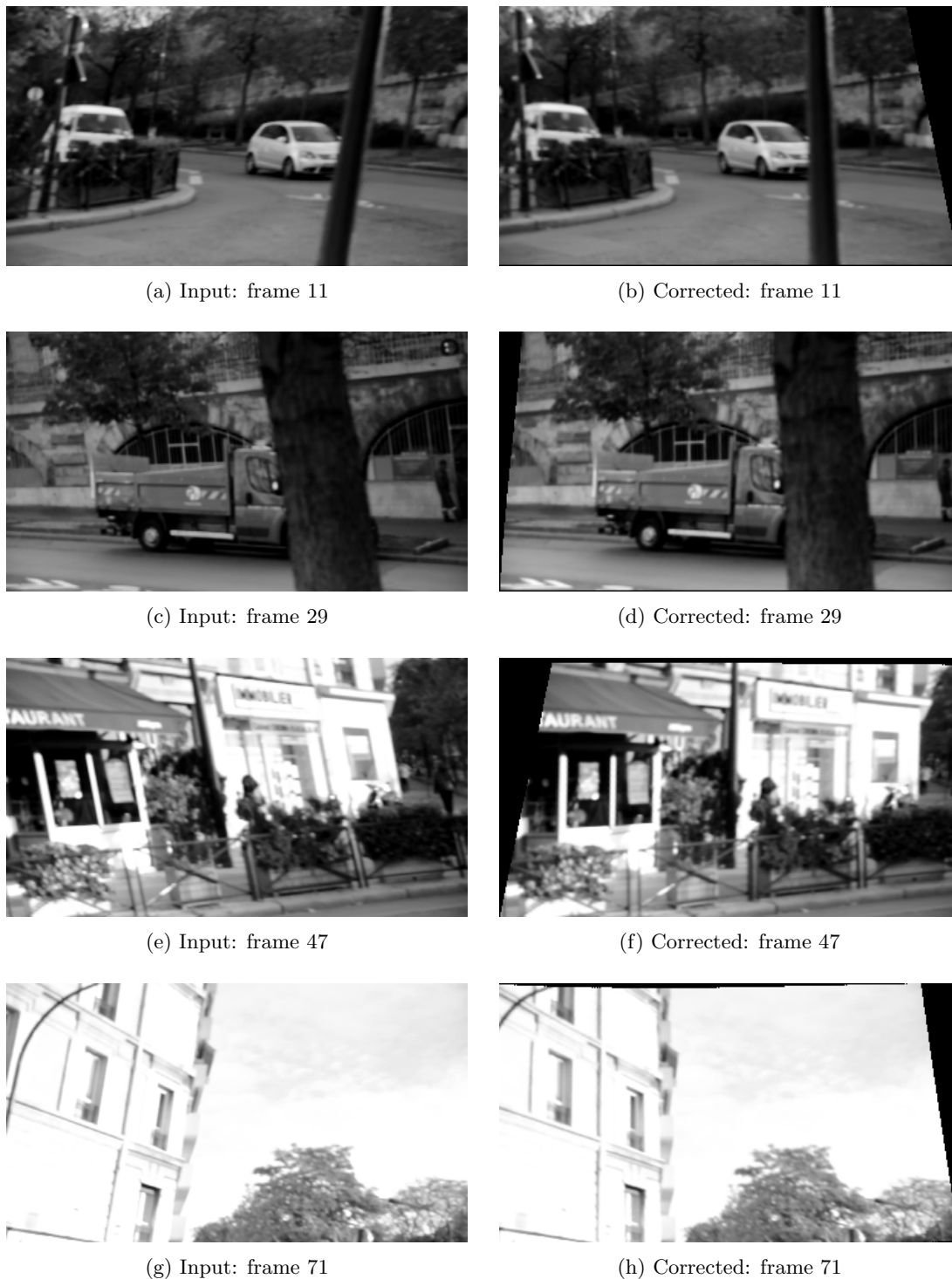
Figure 3.8: Left: input from a true sequence by a fast moving hand-held CMOS camcorder. Right: corrected images. TV-L^1 parameters: 5 levels, 20 global iterations, 5 Chambolle iterations, \lambda = 1.0, \theta = 0.5, \Delta t = 0.125 . Out-of-image warps are displayed in black. Performance: being an old implementation combining OpenCV and GPGPU, approx 1-2 fps.
