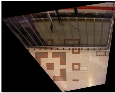
FIG. 9 – Image from S1 (camera 3) transformed by the DLT. In this plane, floor distance can be directly calculated between the bag and owner.
