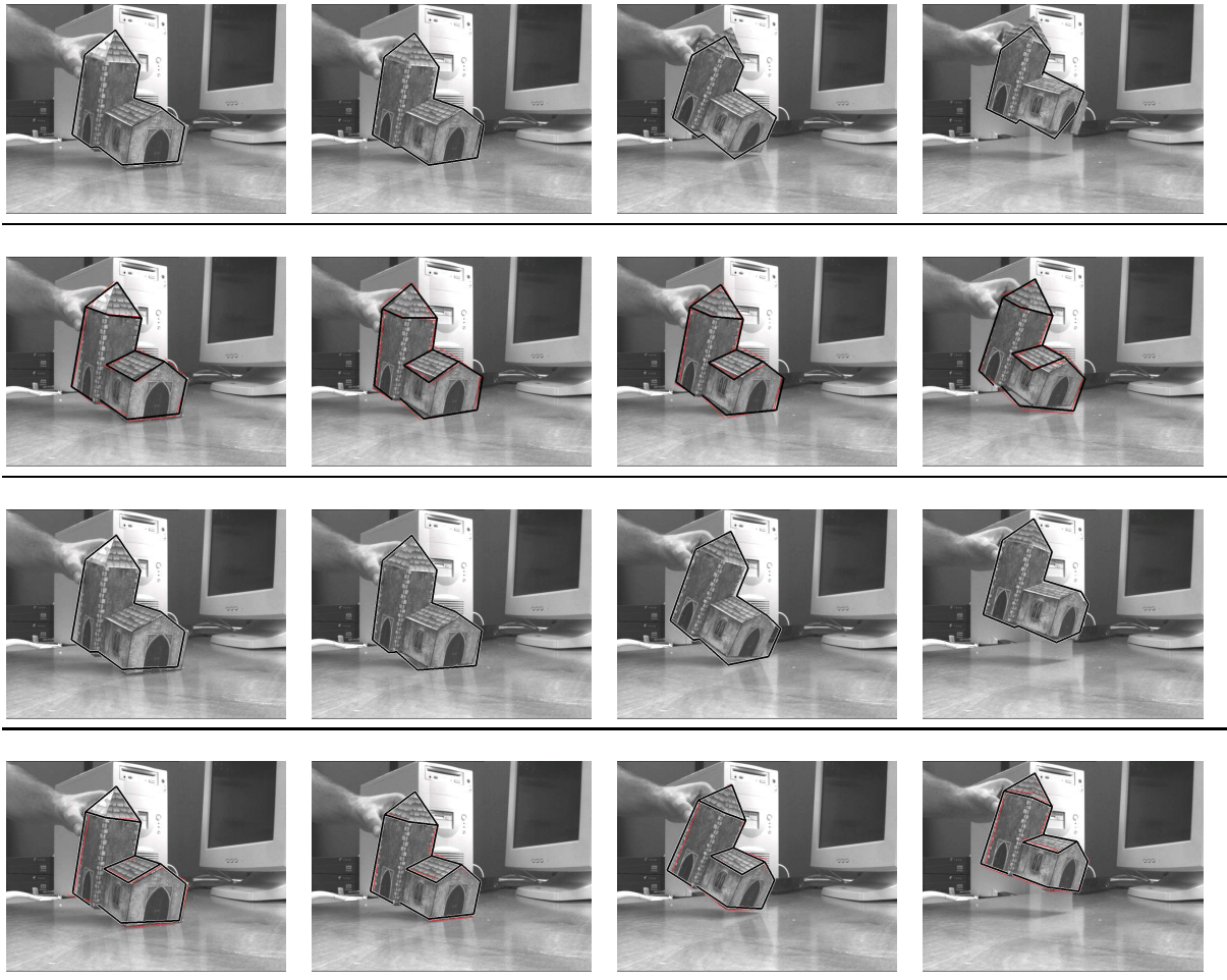
Fig. 10. Comparison between different contour tracking algorithms. First row: Tracking results using an edge-based tracker. Second row: Tracking results using Fisher discriminant function. Third row: Tracking results using Bayesian texture boundary detection and fourth row: Tracking results using the classification-based method.
