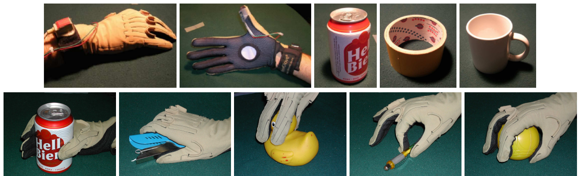
Figure 4: (above) The devices and some of the objects used for the experiment, left to right: the CyberGlove, the Force Resistor Sensor attached to the subject's thumb, the beer can, the duct tape roll and the mug. (below) The 5 grasp types to be recognised, left to right: power large, power flat, tripodal precision, thumb/index precision and spherical precision.
