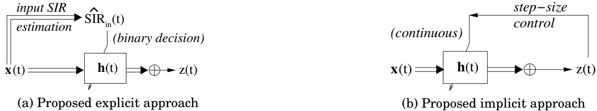
Figure 8.2. Proposed explicit and implicit adaptation control. \mathbf{x}(t) = [x_1(t) \cdots x_{N_m}(t)]^T are the signals captured by the N_m microphones, and \mathbf{h}(t) = [\mathbf{h}_1(t) \cdots \mathbf{h}_{N_m}(t)]^T are their associated filters. Double arrows denote multiple signals.
