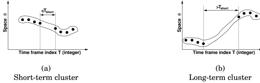
Figure 6.3. The two types of clusters. This chapter focuses on short-term clusters (a), obtained with location cues only. Long-term clustering (b) requires additional cues, as investigated in Chapter 7.
