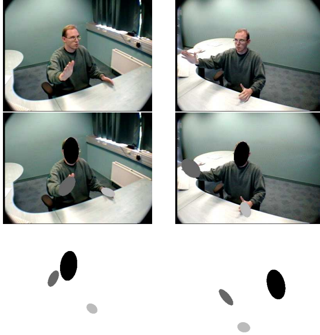
FIG. 4.5 – Top : left and right captured images. Middle : left and right images with projected ellipsoids. Bottom left ellipsoids projection on the frontal plane. Bottom right : ellipsoids projection on the side plane (the cameras are on the left side)
