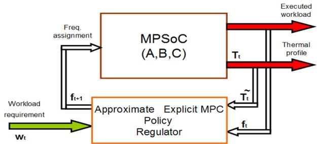
Fig. 1. Diagram of proposed approximate-explicit-MPC-based thermal management policy
