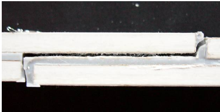
Figure 5. Typical failure mode of SLJ with same-side crack pattern.
