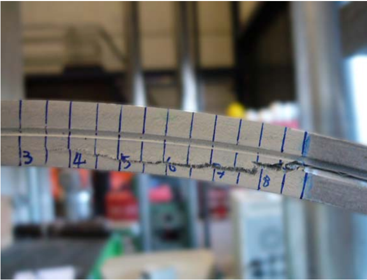
Figure 8. Failure mode of ELS01 (crack in roving layer).
