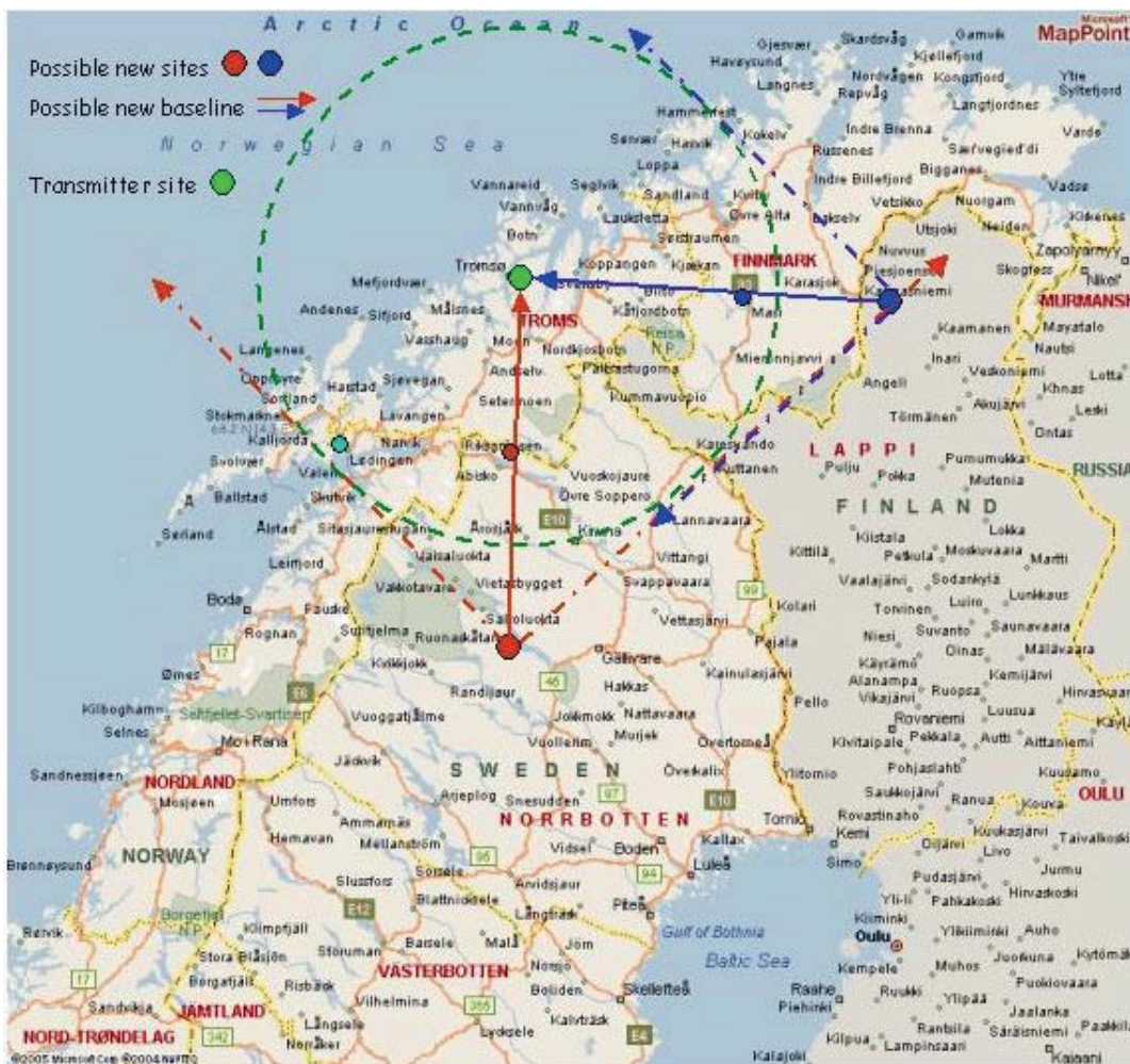
Figure 1. A map of the deployment area of the projected EISCAT_3D radar system, showing the locations of the antenna sites. The dashed circle indicates the approximate extent of the common field of view at 300 km altitude.
