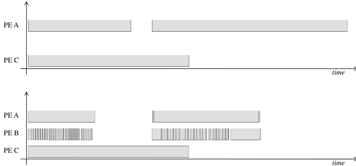
Figure 7. 2-PE (top) and 3-PE (bottom) schedules for the hybrid block operation mode.
