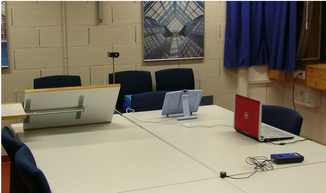
Figure 9.7: Workplaces of the CLC Exposure Room. - Photograph of the two workplaces in our CLC Exposure Room, with the reading/writing supports, the digital spectroradiometer as well as a luxmeter that is used to continuously monitor the horizontal workplane illuminance in the center of the room
