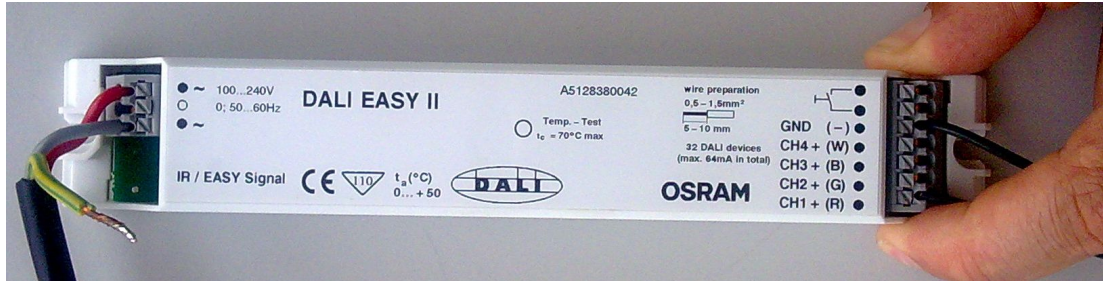
Figure 5.3: DALI Easy II lighting control unit. - The figure shows the DALI Easy II lighting control unit installed in the test office room of the LESO building.
