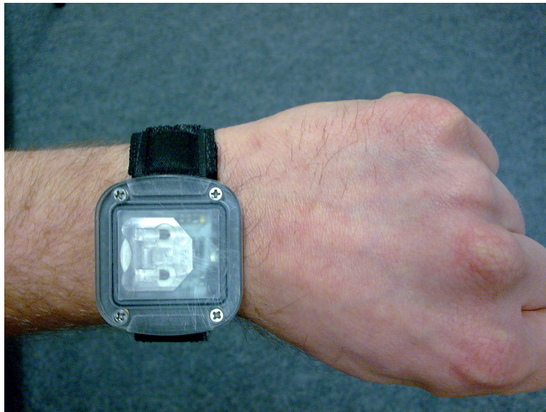
Figure 9.6: The Daqtix device. - Study participants wear the Daqtix® seven days prior to the study at their non-dominant wrist. The device records acceleration values and illuminances.
