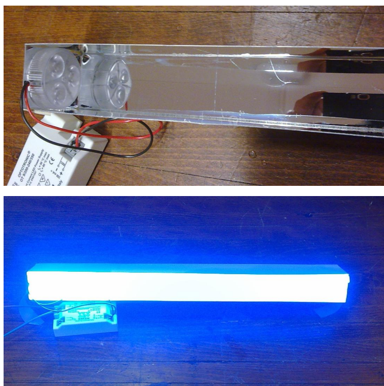
Figure 8.6: The BlueLum prototype. - The Figure shows photographs of the luminaire and the mounted blue LED device (top) and the luminaire covered by the paper screen switched on (bottom).
