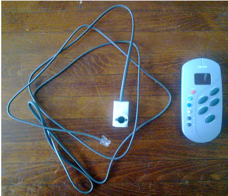
Figure 5.5: Infrared sensor and remote control. - The figure shows the remote control as well as the IR receiver connected to the DALI controller.
