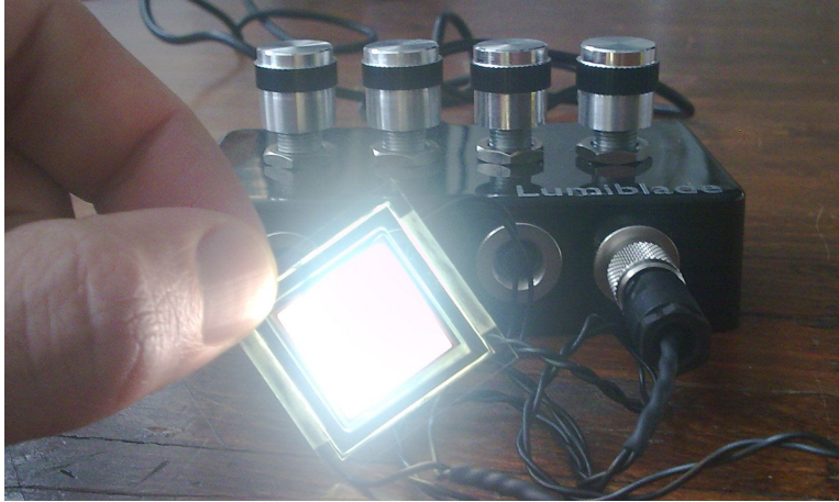
Figure 3.10: White OLED. - White Lumiblade OLED "Pixel" in operation at the LESO-PB.
