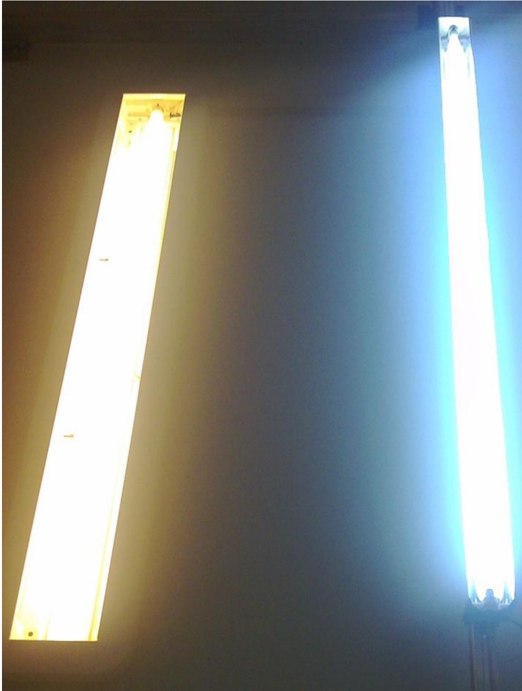
Figure 7.2: Warm white light and blue-enriched white light. - This Figure visualizes the difference between a warm white fluorescent tube and a blue-enriched fluorescent tube as used during the study by Viola et al. (111).
