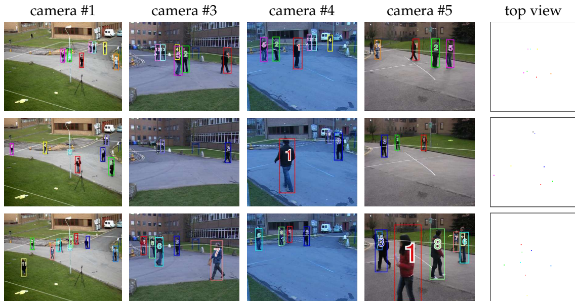
Figure 4.16: Multi-camera pedestrian tracking results on the PETS 2009 data set. Each of the first four columns shows a different camera view. The fifth column displays the top view.
