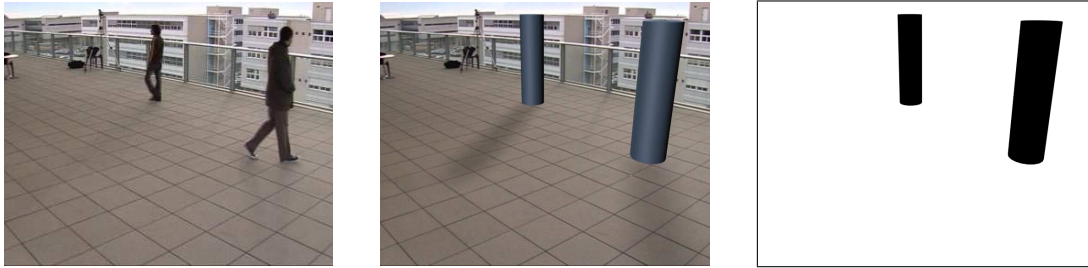
Figure 2.3: This figure illustrates how the space occupied by pedestrians can reasonably well be approximated with cylinders of 50 cm diameter and 1.75 meter high. The right image shows that the cylinders projection in the image plane is close enough to vertical rectangles, when the camera is located sufficiently low relatively to the ground.
