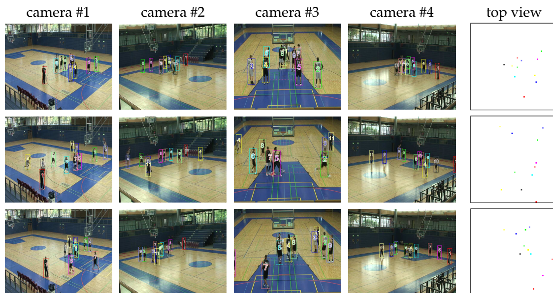
Figure 4.14: Multi-camera pedestrian tracking results on the basket video sequence. Each of the first four columns shows a different camera view. The fifth column displays the top view.
