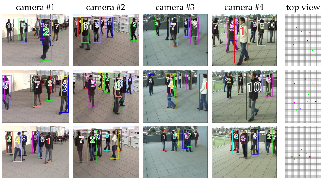
Figure 4.13: Multi-camera pedestrian tracking results on two video sequences of the terrace data set. Each of the first four columns shows a different camera view. The fifth column displays the top view.
