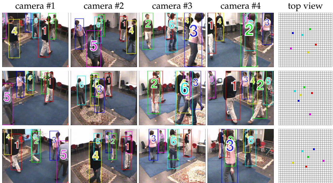
Figure 4.3: Tracking results on the laboratory sequence. Each row displays several views of the same time frame coming from different cameras.
