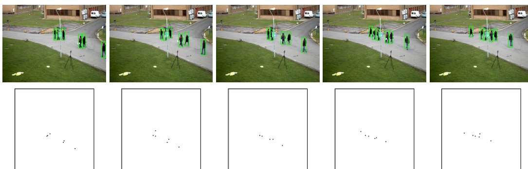
Figure 3.14: Monocular detection results on the PETS 2009 sequence. The first row shows camera view bounding boxes at different frames, while the second row displays the occupancy maps.
