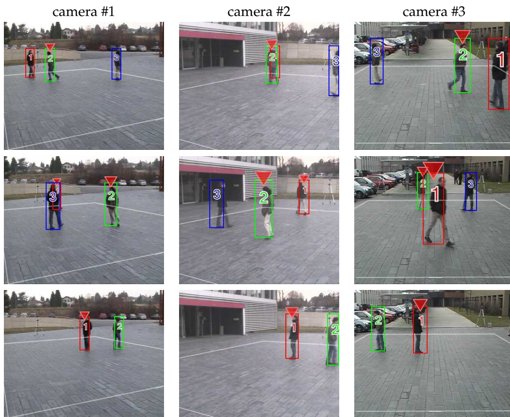
Figure 5.12: Anomaly detection in camera views. Each row consists of views from three different cameras at the same time frame. A red triangle above a person indicates that it does not move according to the learned model.
