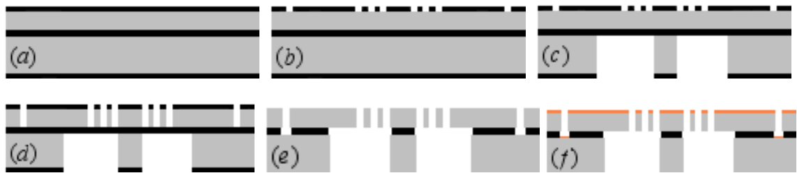
Figure 3.6: Schematic of the process flow (not to scale). (a) LPCVD SiO 2 . (b) Topside lithography and RIE. (c) Backside lithography, RIE SiO 2 and DRIE. (d) Topside DRIE. (e) SiO 2 etching in HF vapor. (f) E-beam evaporation of Cr and Au on topside.
